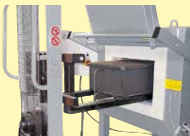
Working with protective gas boxes for a protective gas atmosphere using a charging cart
