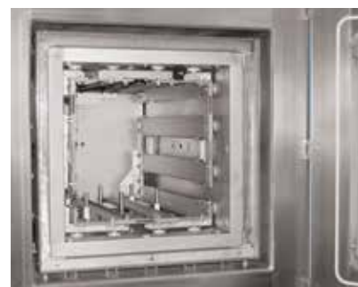
Molybdenum or tungsten heating chamber
