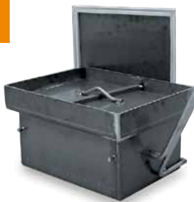
Protective gas box for N 41/H furnace with additional evacuation lid
