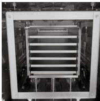
Molybdenum inner process chamber incl. six charge supports
