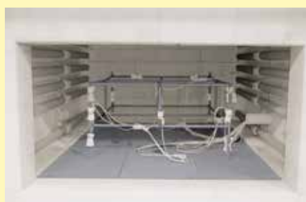
Measurement set-up in an annealing furnace
