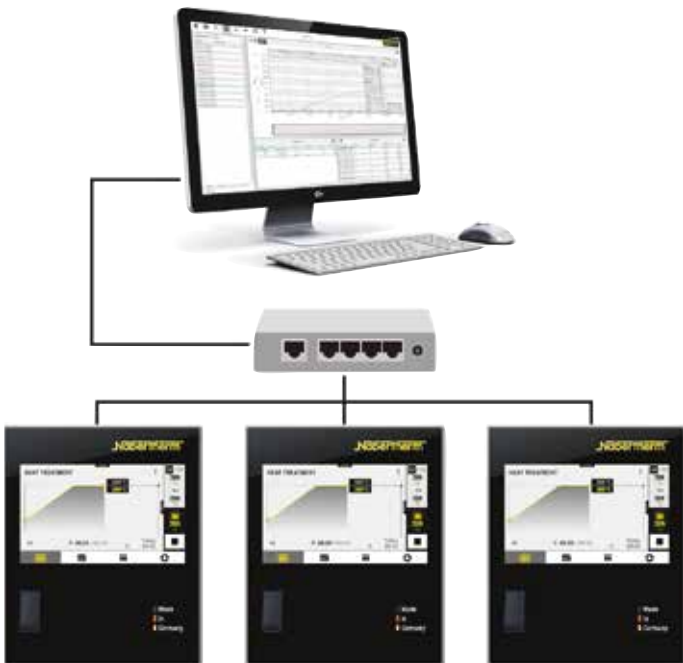
Example lay-out with 3 furnaces
